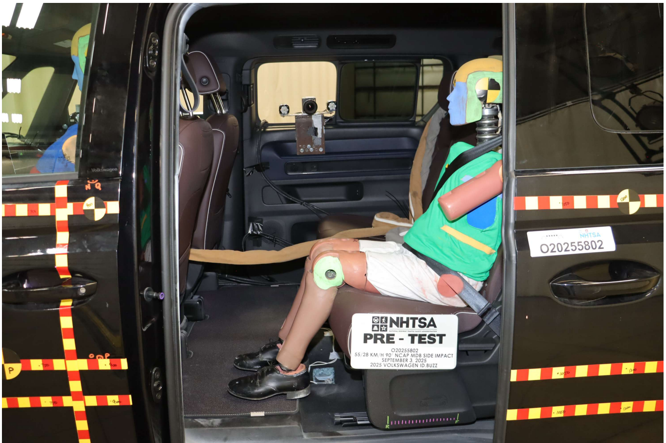
Photo No. 055 - Pre-Test Left Side View of Rear Passenger Dummy Showing Belt and Chalking
