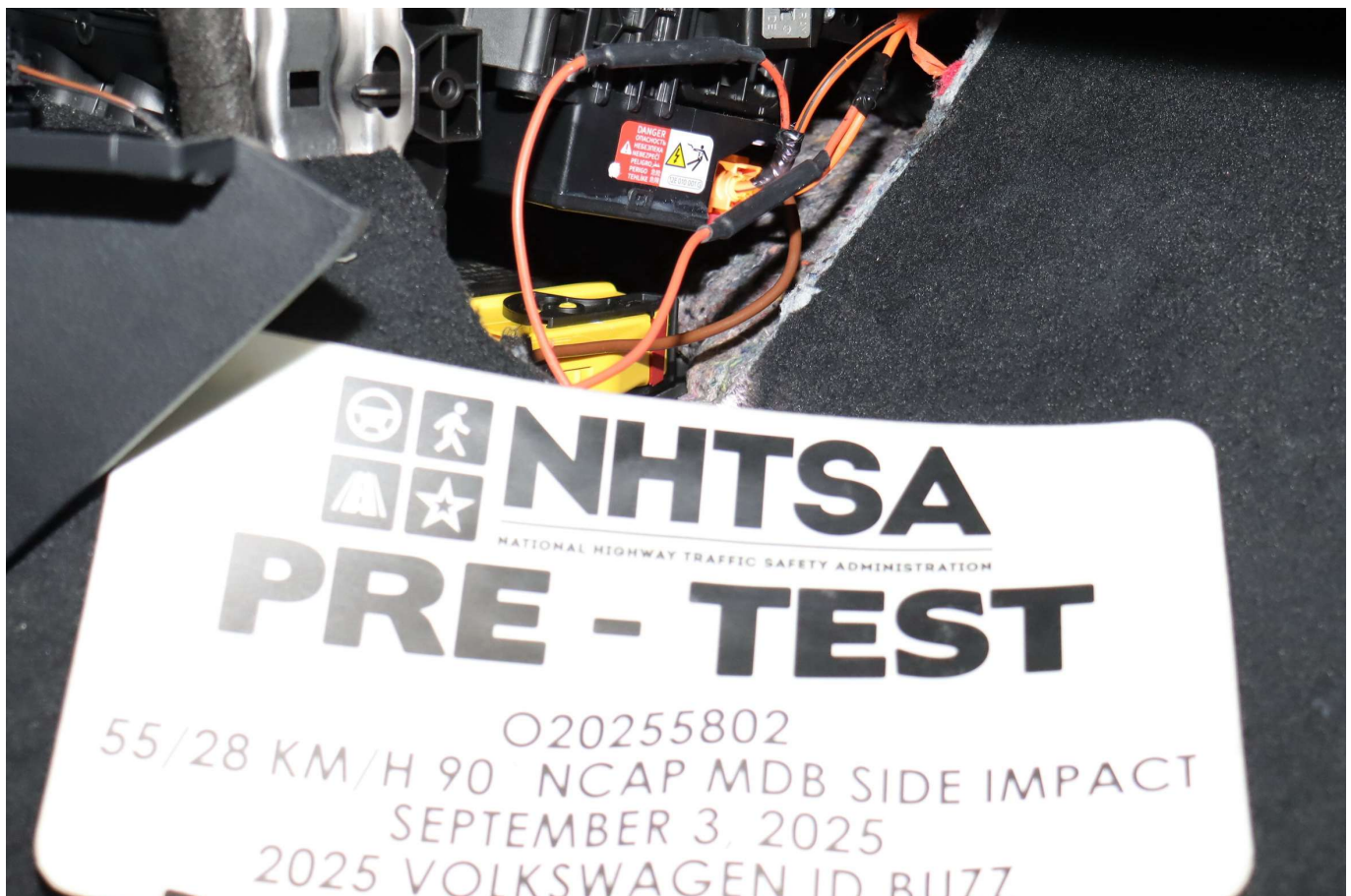
Photo No. 305-02 - Power Inverter Warning Label
