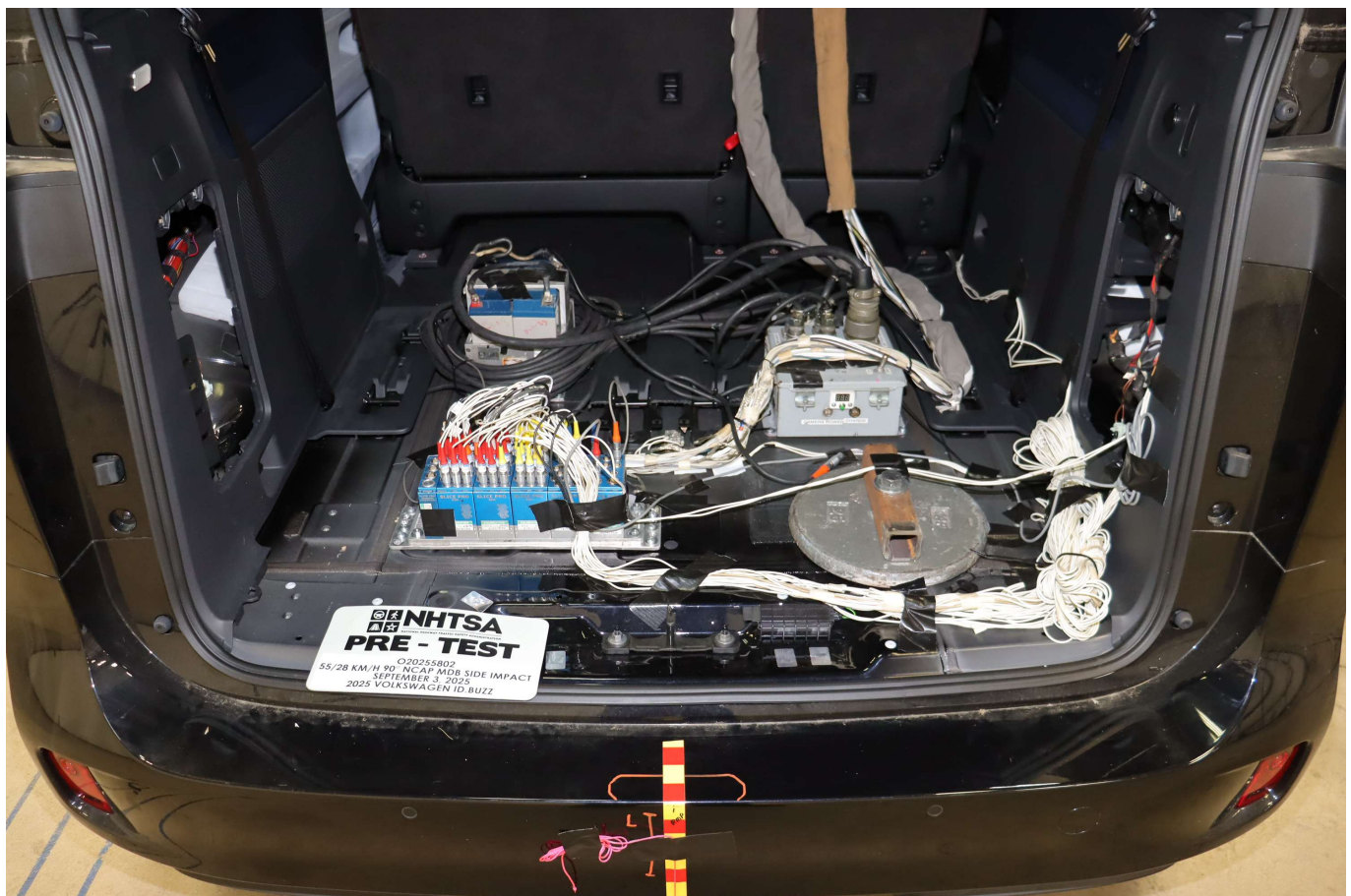
Photo No. 094 - Pre-Test Ballast View
